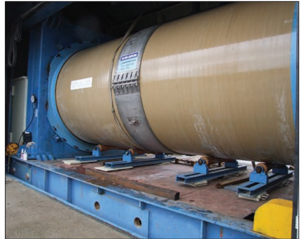
▲ HYDRO PRESSURE TEST( \phi 2,860 )
