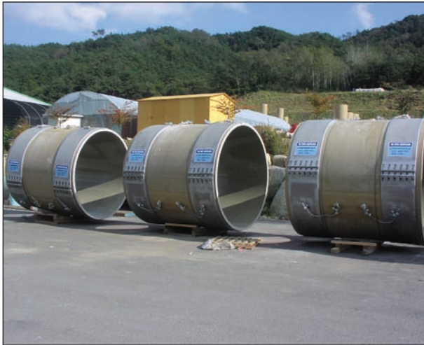
▲ LARGE WATER SUPPLYING PIPELINES(2,800mm)
